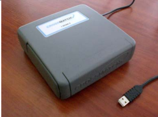
Figure 10: Double Iris Capturing Device with USB Connector (Model 1)
